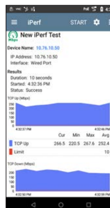
iPerf throughput test with TCP or UDP frames
