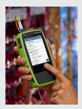
The EtherScope<sup>™</sup> nXG is a portable network expert, easy to use for network technicians, but powerful enough for network engineers. As a multi-technology, all-in-one handheld network analyzer, it enables engineers and technicians to get more done faster, from deployment to maintenance, troubleshooting, and documentation of their ever-changing Wi-Fi and Ethernet access networks.
