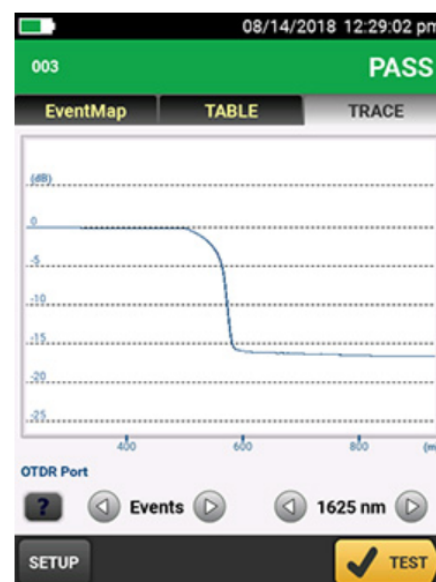
Splitter as seen on an OTDR trace
