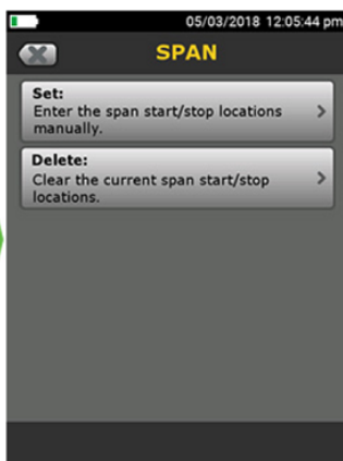
Process to set Span on an OptiFiber Pro OTDR
