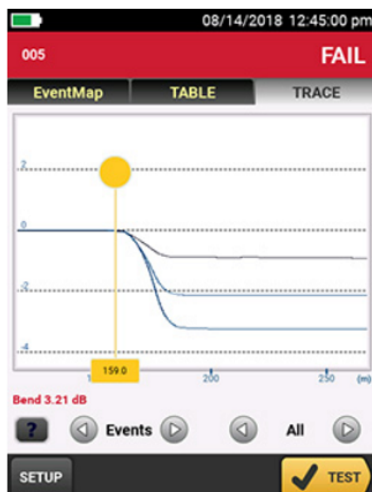
Bend as seen on an OTDR trace
